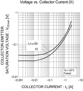
Fig.6 Collector-Emitter Saturation
